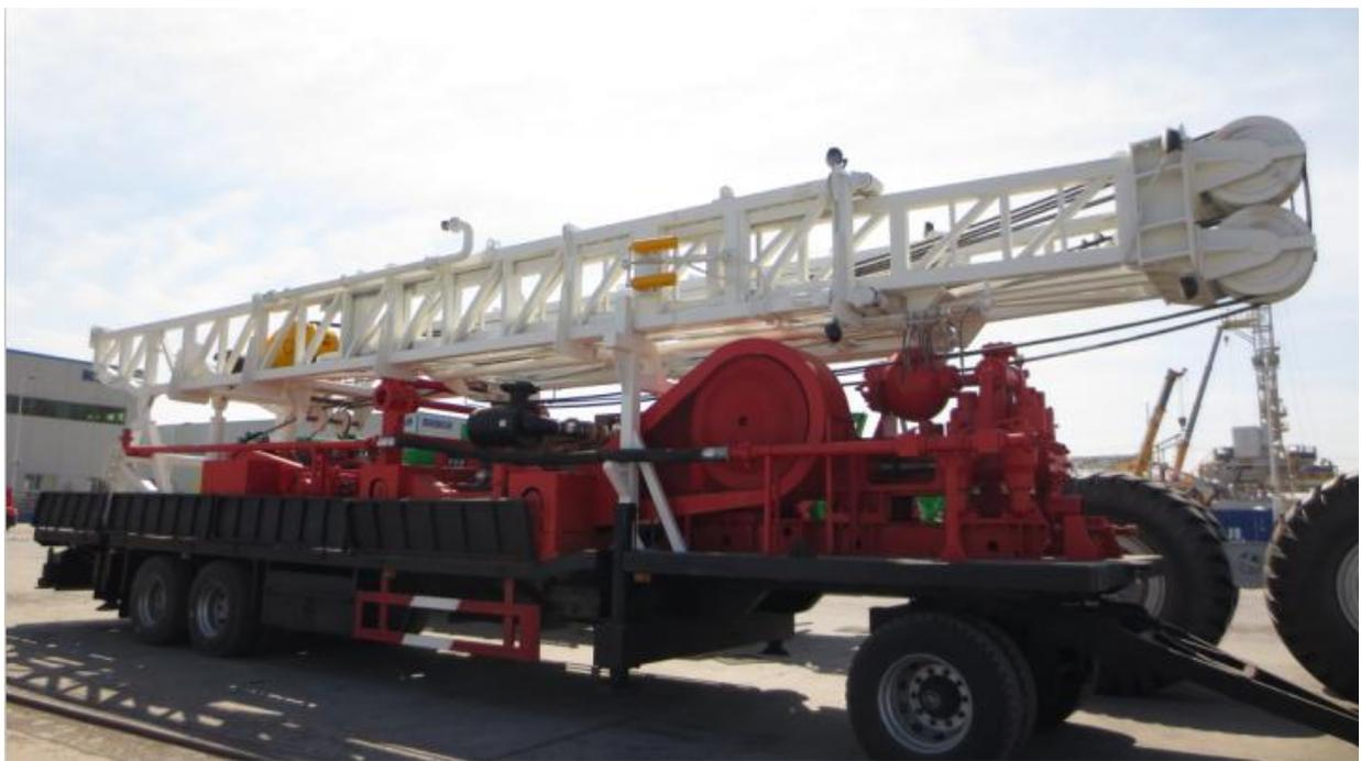
1 This drilling rig is one type of normal-circulation rotator. The chassis of full-trailers is applied in this drilling rig which is being equipped with all-steel meridian tires with good off-road performance.
